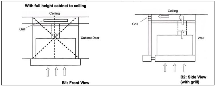
Installation: Ventilation Airflow for Telescopic hood AT1349 (with grill)
